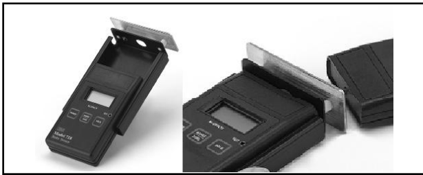
Figure 6. 718 Static Sensor charging plate in use.
