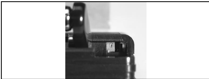
Figure 9. 718 Static Sensor adjustable screw for display.
