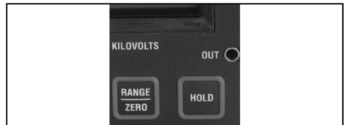
Figure 5. 718 Static Sensor has a continuous output range.
