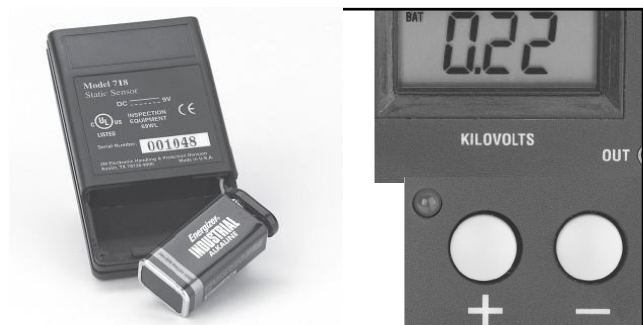
Figure 2. SCS 718 and 718A Battery Replacement and Indicators.
